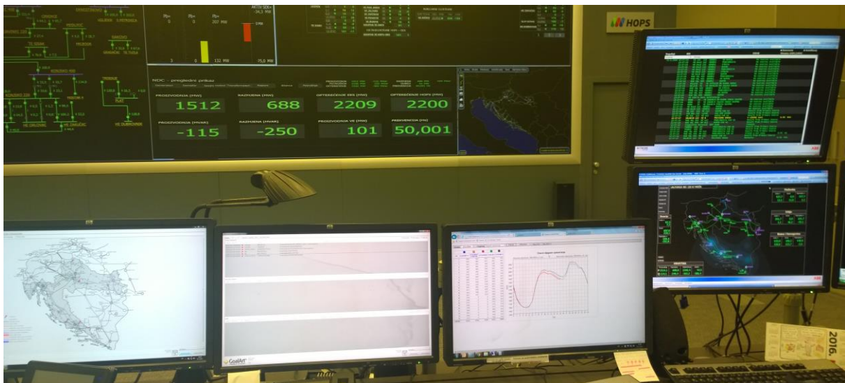
Figure 1. An operator workplace. The IAP tool is on the two left bottom screens (graphical overview and alarm list with root alarms and secondary alarms). The lightning detection tool is on the bottom right of the video wall. The smart visualization of voltage deviations is on the bottom screen on the far right.
